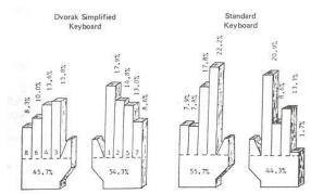
In this figure, the lengths of the fingers are proportional to the work each one does.
