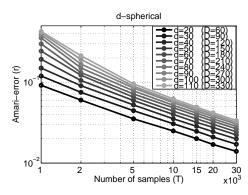
Figure 4: Estimations of database *d*-spherical: Amarierror as a function of the number of samples on loglog scale for different dimensional (*d*) subspaces. Task dimension: *D*. Errors are approximately linear, so they scale according to power law, like  $r(T) \propto T^{-c}$  (c > 0). For numerical values, see Table 2.
