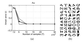
Figure 3: Estimations on database  $A\omega$ . (a) Amari-error as a function of the number of samples. Average±deviation for 30000 samples:  $0.58\% \pm 0.04$ , (b) estimation with average error for 30000 samples: the hidden components are recovered up to permutation and orthogonal transformation ( $\mathbb{R}$ -ISA ambiguity).
